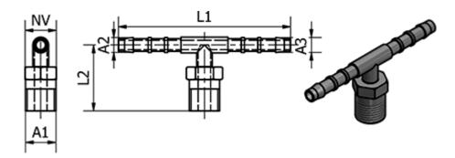
Ext. hose diameter A2 = 6Ext. hose diameter A3 = 6L1 = 57 L2 = 26 NV = 14 Thread A1 = R 1/4"
